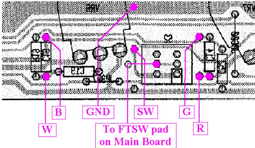
This diagram shows how the wires from the Tone Stack and Boost Switch hook up to the add-on relay board.
