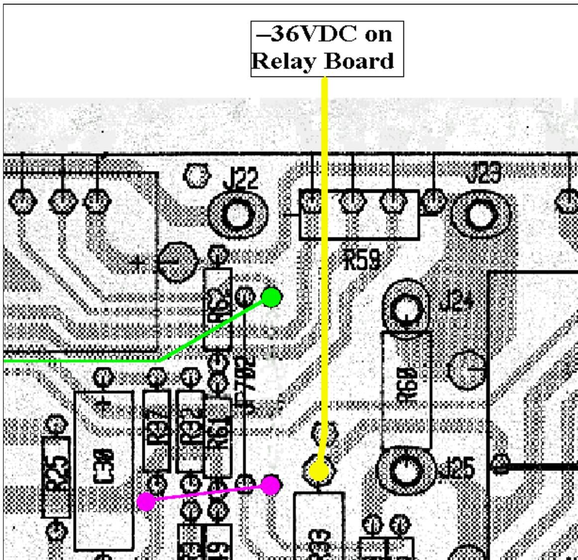
This drawing shows the connections for the relay board and footswitch on the main board (component side):
