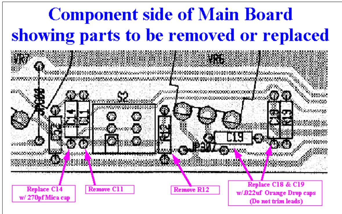
As the diagram indicates, you need to remove C11 and R12. If you haven't done so already, you should replace the C14 Treble cap with a 270pf/500V mica cap, and both C18 and C19 with high quality .022uf caps. While I used 600V Orange Drop caps, you might like to try 630v metallized polyester caps for a brighter, clearer sound. Leave the leads for the C18 Bass cap uncut as you may want to use them for flying leads up to the add-on relay board.
