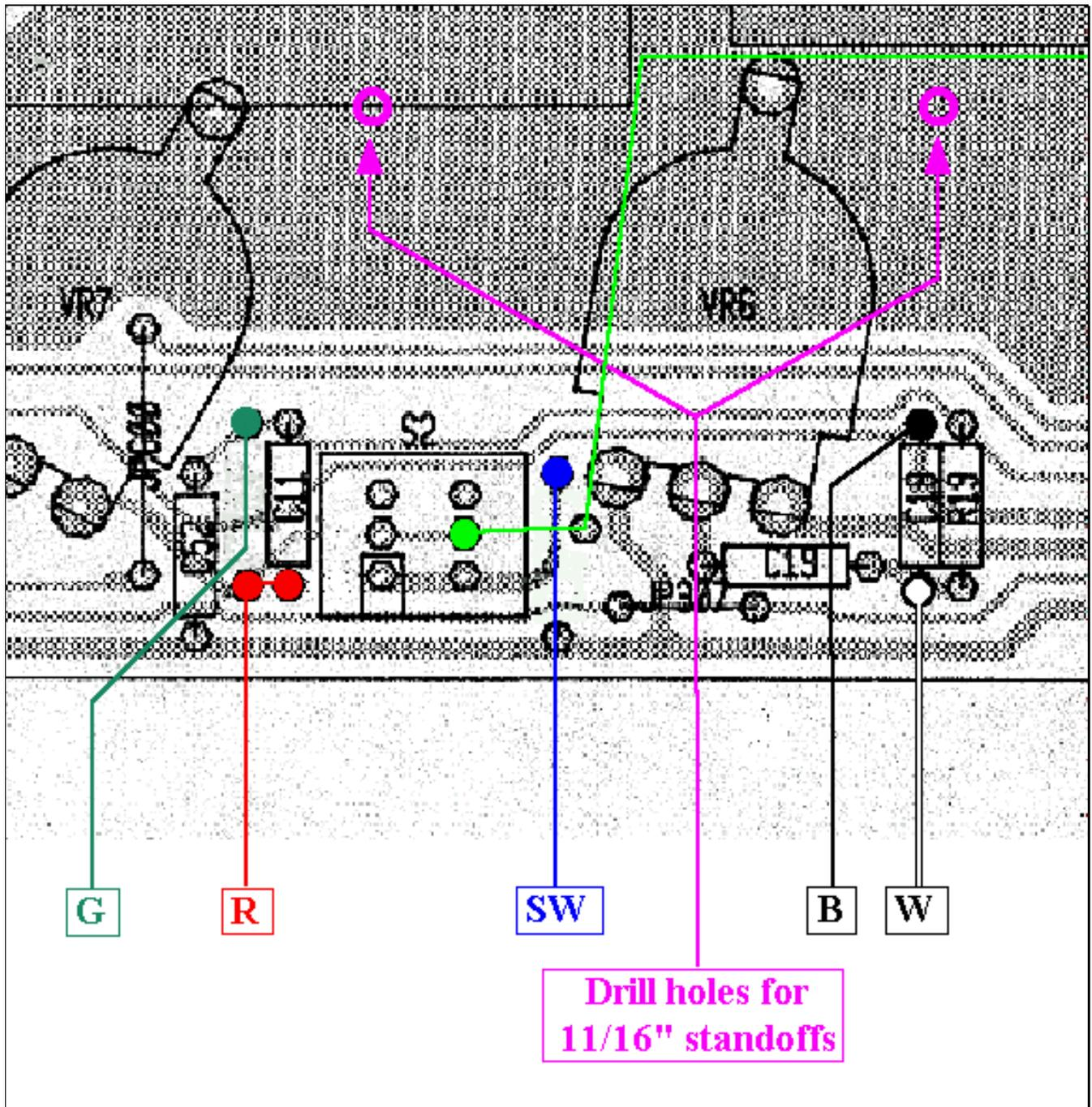
This drawing shows the Tone Stack/Boost Switch section of Main Board (component side):
